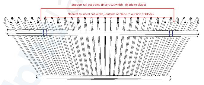
Now take the difference in measurement between insert cut width and the outside to outside of blade and divide it by 2. This measurement difference is how far to cut into the support rail for a centred section.
