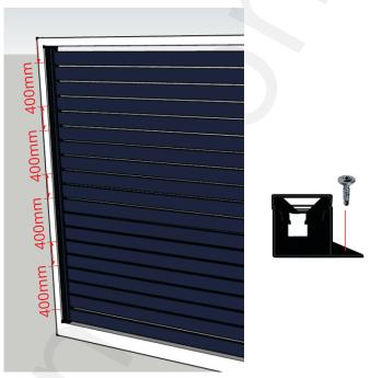
Install the complete slat assembly into the gate with the Flat area of the F channel to the inside of property. Make any adjustment now for the width using a rubber mallet. Fix in place from the back side of the flat section using wafer head screws.
