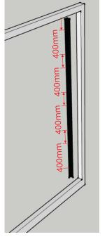
Install the angle inside the gate frame with the open side towards the street (ready to accept the slat system).
