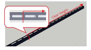
Cut ALL pre-punched channels to the internal clear height.
