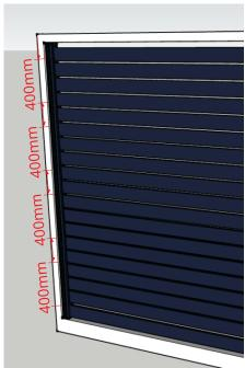
Install the complete slat assembly into the gate. Make any adjustment now for the width using a rubber mallet. Fix in place from the back side of the angle using wafer head screws.
