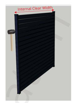
Now tap the OTHER pre-punched channel onto the slats ensuring not to cause damage and facing the punched channels CUT in the same direction as the first channel assembly installed.
