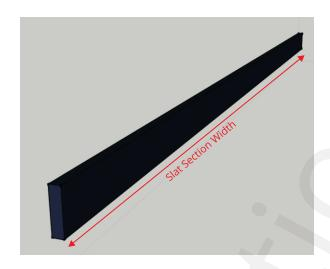
Cut ALL slats to the "Slat Section Width" appropriate to the gate size.
