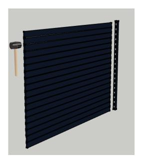
Using a rubber mallet tap in all the slats into the first pre-punched channel. Ensure to carefully TAP slats into place ensuring not to damage the ends.
