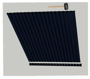
Using a rubber mallet tap in all the slats into the first pre-punched channel. Ensure to carefully TAP slats into place ensuring not to damage the ends.
