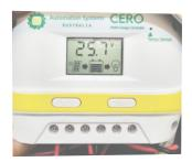
The Cero Solar Regulator by default is Auto-Detecting for the voltage setting and battery type, **no changes to its menu settings are required.**
