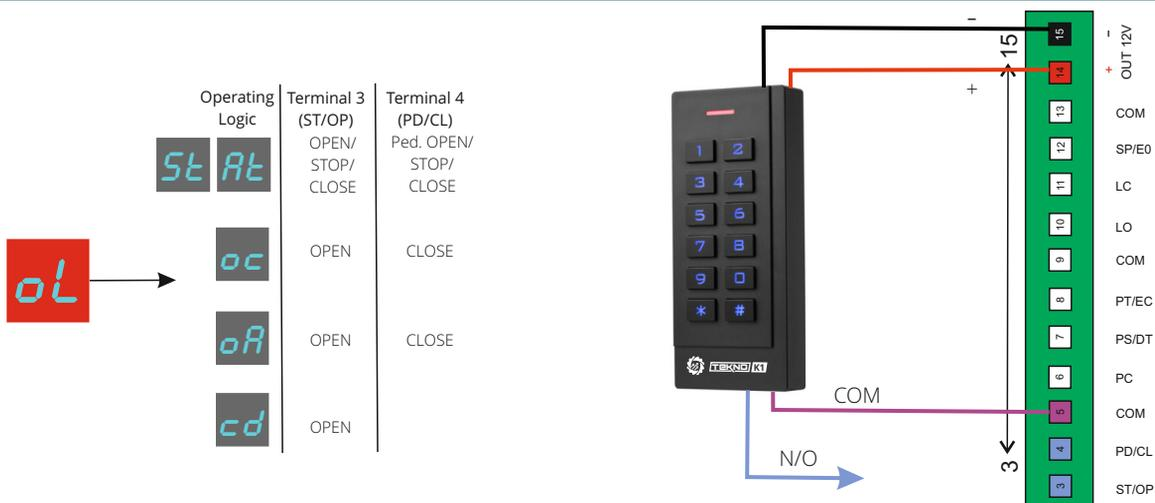
For Full Gate operation OPEN and CLOSE connect to terminal **START 19**
