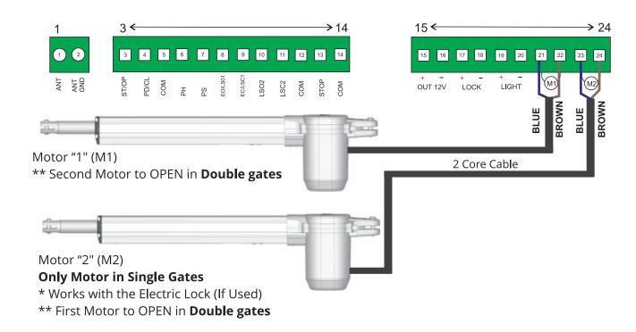
Follow the Premier SW24 Instructions for setting the control board with series limit to be defined as (NT). Furthermore if required set the system to single gate if only one motor unit is in use (YS). These settings are all located in the advanced menu of the control board.
