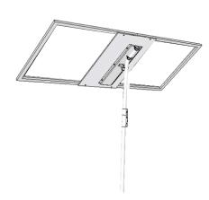
6. Install to fence post or pier using the supplied pipe clamps.
