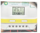
The Cero Solar Regulator by default is Auto-Detecting for the voltage setting and battery type, **no changes to its menu settings are required.**
